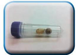
Load tube with sample (dry corn kernel) and ceramic ball.
